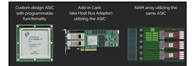
There is the CXL/Gen-Z converter and switch ASI implemented on a host adapter card that can be used as an endpoint in a server and a network attached memory (NAM) appliance, shown on the right.
