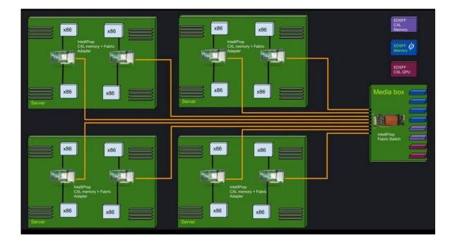
The neat thing about external memory servers is that the CXL-Gen-Z fabric that IntelliProp has created doesn't care if the physical memory on the other end of the 802.3 wire is DDR3, DDR4, DDR5, or HBM stacked DDR memory. The latencies and bandwidths will play out as they do, but customers could choose very cheap memory or the very expensive stuff, depending on their capacity and bandwidth needs, out there on the memory appliance.
